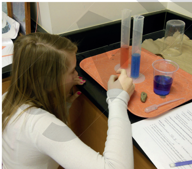
Figure 1.6: A student measuring the volume of a liquid. Her eyes are level with the scale so that she can accurately measure where the meniscus meets the scale.
