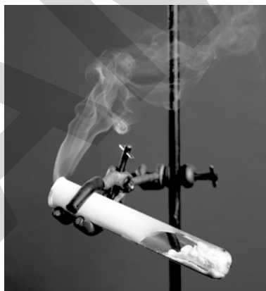
Figure 1.7: Sublimation of ammonium chloride.
