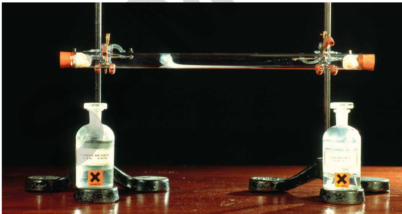
Figure 1.21: Ammonia and hydrochloric acid fumes diffuse at different rates.
