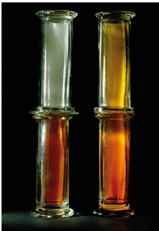
Figure 1.20: Bromine vapour diffuses throughout the container to fill the space available.
